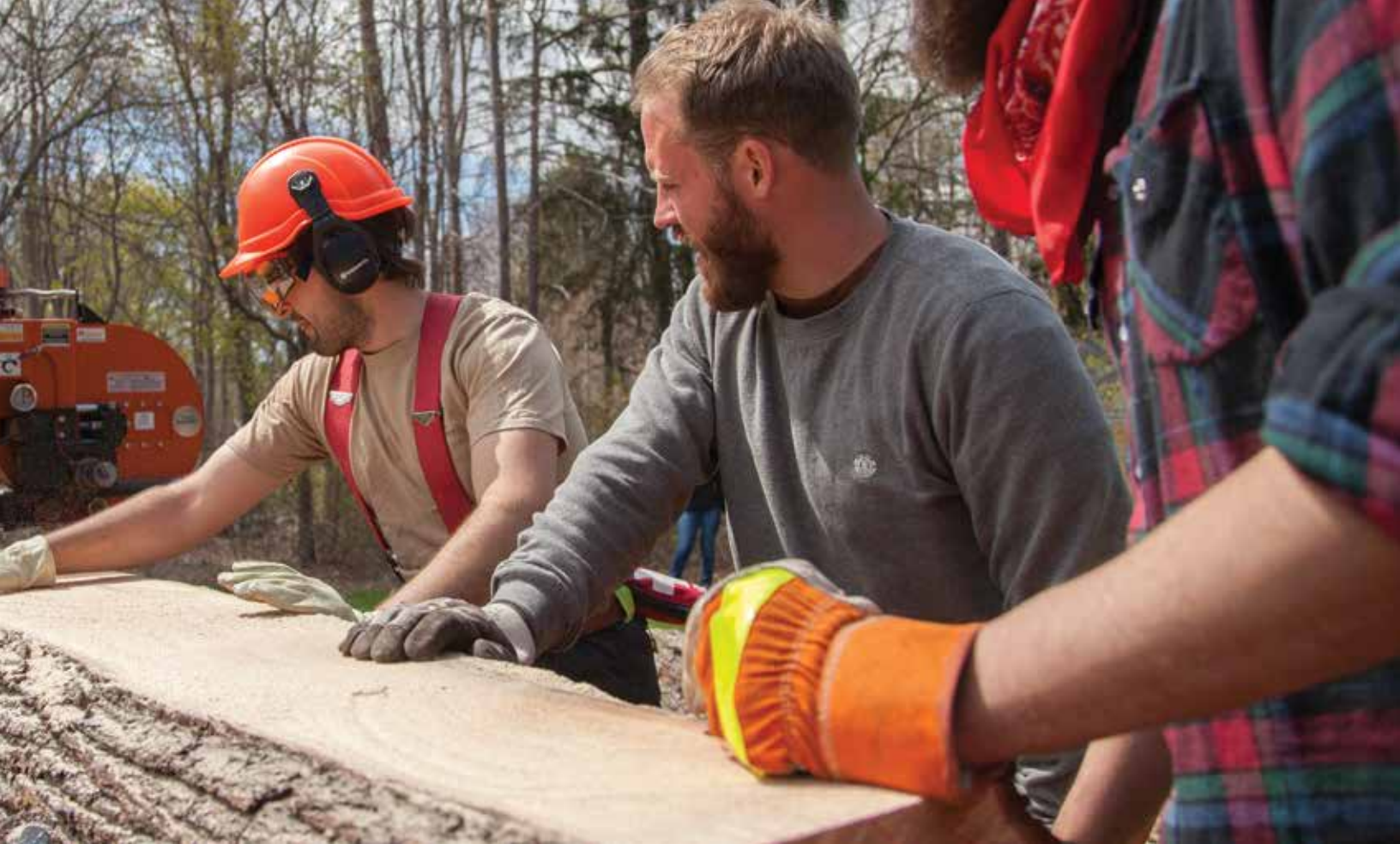
Above: Sean Mahoney of Mass DCR and David Kennedy and Jacob Mans of Decentralized Design Lab use a portable saw mill to cut boards from a red maple log harvested on Prouty Woods.
