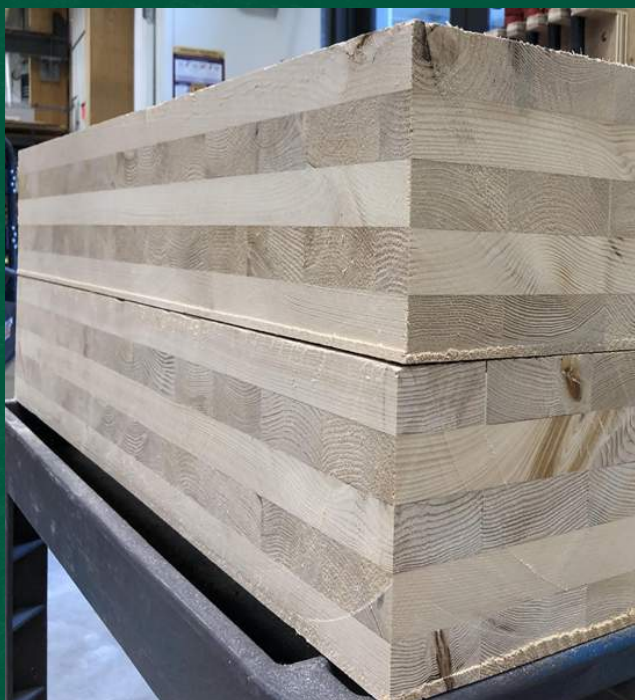
5-layer Eastern Hemlock CLT panel fabricated in University of Massachusetts Amherst's Wood Mechanics Lab. Image courtesy of Peggi Clouston.
