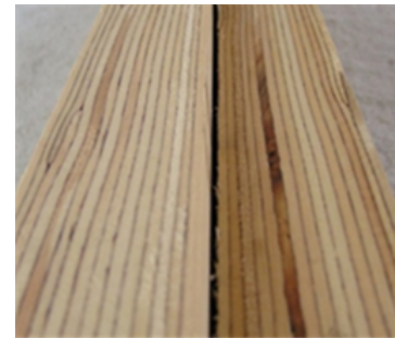
LVL layered structure
